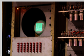
Figure The CRT output showing the memory contents as a matrix of 32 × 32 big/small dots (credit: Wikipedia)
