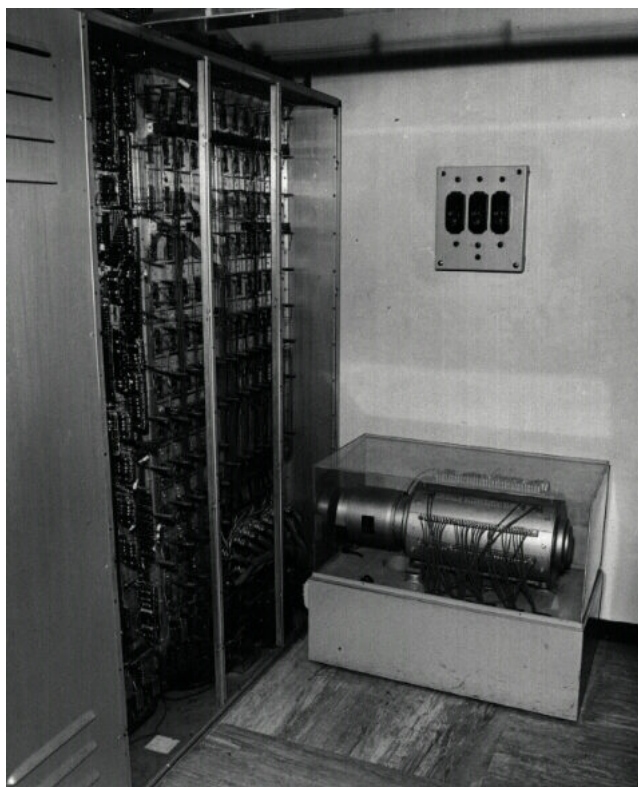
Figure 1: The magnetic drum memory of the CEP, 1961. It has a capacity of 16384 36-bit words. (credit: www.cep.cnr.it ).
